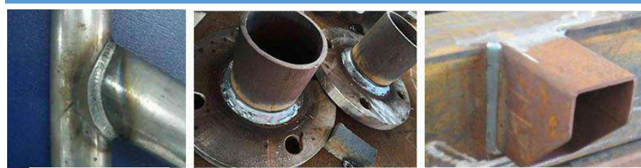
Tube Welding Round Welding Square Tube Welding
